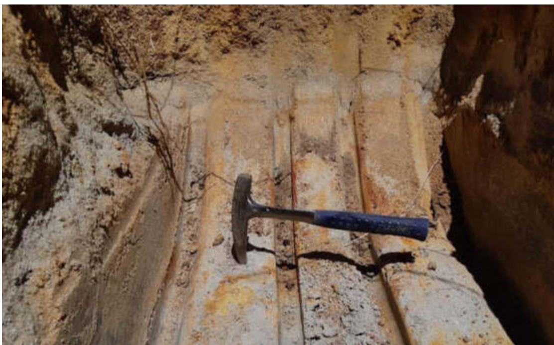
Figure 32: TP10 – Close up of bottom of trial pit; note sidewall smear near base of trial pit.
