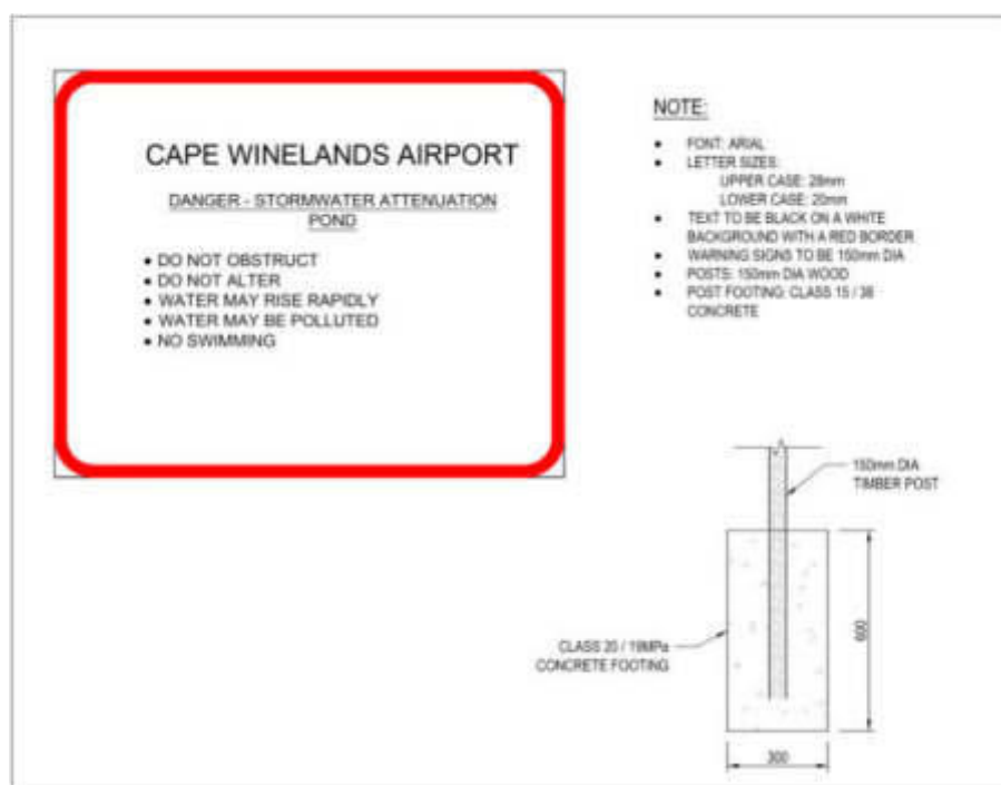
Figure 33: Typical Stormwater Pond Safety Signage
