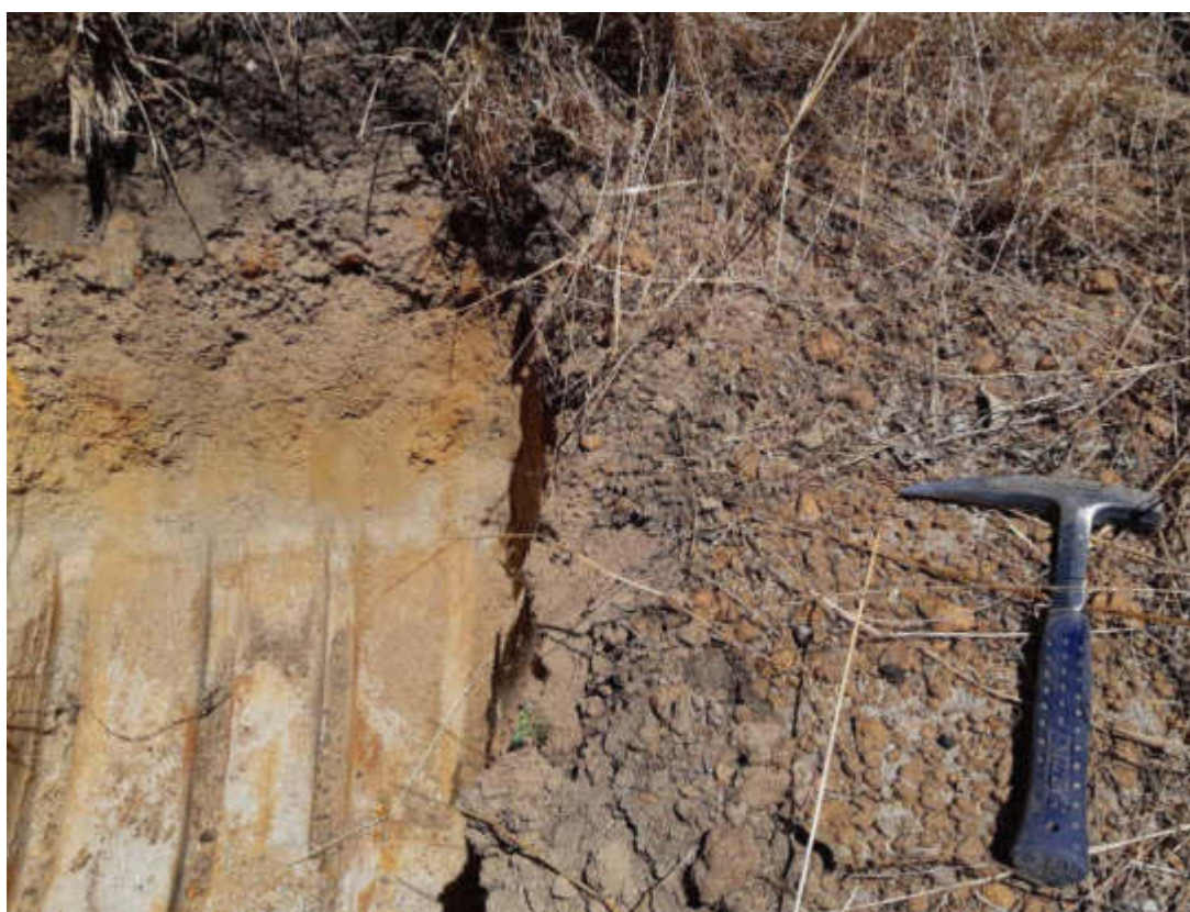
Figure 33: TP10 – Close up of bottom of ferricrete nodules strewn across surface surrounding trial pit; exposed soil profile pictured on LHS of photograph.
