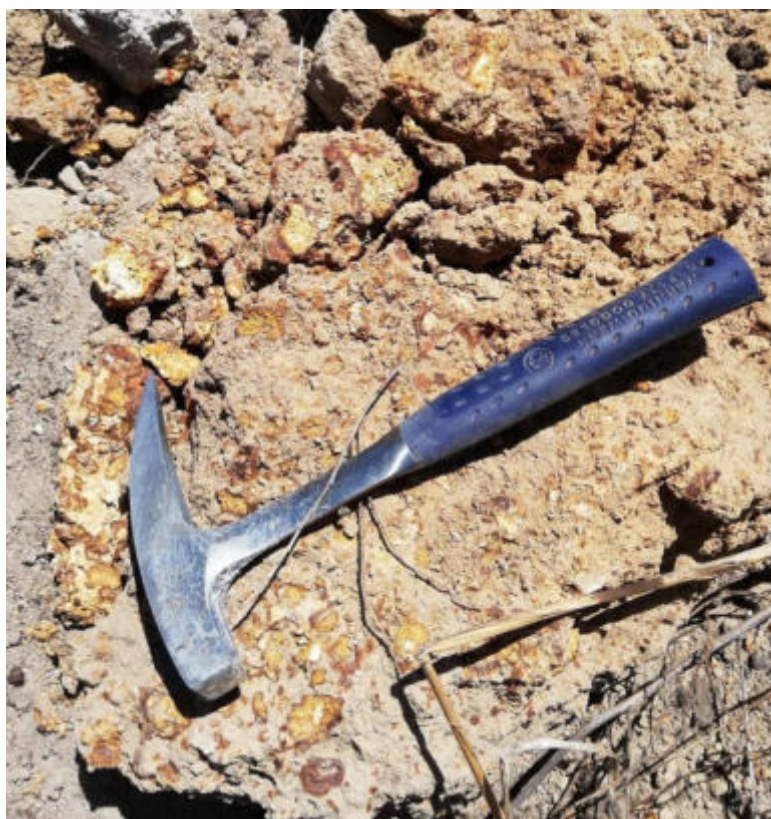
Figure 49: TP28 – Ferricrete boulders (approx. 300 mm in diameter) excavated from pedogenic hardpan ferricrete horizon.
